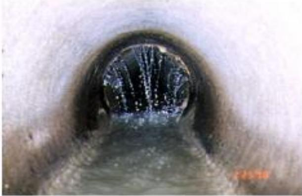
**Dyed Water Testing** will be conducted in some areas. A rainfall like test using biodegradable and nontoxic fluorescent dyes will help detect inflow and infiltration into the sewer system. The dyed water is placed in downspouts, area drains, and low lying lawn areas to identify sources that are deteriorated, broken, or incorrectly connected to the sewer system.
